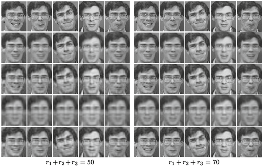
Fig. 5 Recovered images for the ORL database of faces [rows from the top to the bottom: 1. Original, 2. Algorithm 3, 3. ALS (the best), 4. ALS (the worst), 5. Algorithm 2]
